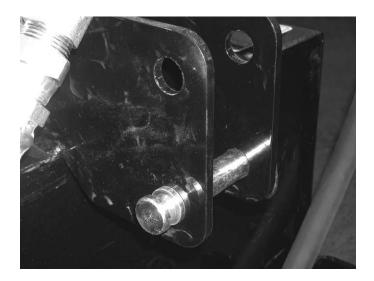
9. Set-up assembly of the pump is now complete. See "Mounting Instructions" on pages 12-13 for instructions on mounting the tank to the tractor for operation. Be sure to check that all fittings are tight after mounting the PTO pump for the first time.
