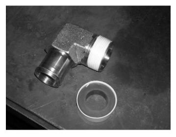
3. Apply Teflon thread tape to the #24 NPT elbow as shown.
